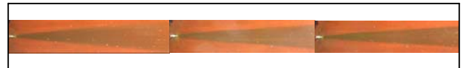
Figure 4.25: SSLC results for the turbulent wedge under zero, mild and strong (favourite) pressure gradients respectively [4.28].
