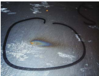
Figure 6 Heated sign on the top surface between guide vanes
