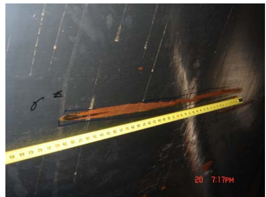
Figure 10 A representative damage-strip showing wedged head
