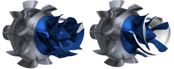
Fig. 13 Regions in the impeller with void fraction over 90%. Pump with axial diffuser, \phi/\phi_{BEP}=0.55 . NPSH \approx NPSH3 (left), NPSH \approx NPSHb (right)
