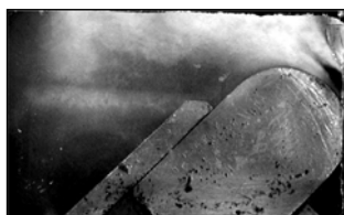
Visualization of cavitation (upstream pressure 12 bar, downstream pressure 1.2 bar, slot width 5 mm)
