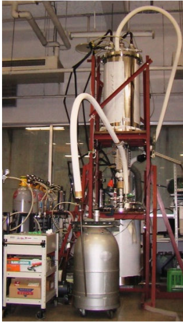
Cavitation tunnel for either liquid nitrogen and water
