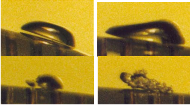
Figure 12. A series of photographs illustrating, in profile, the growth and collapse of a traveling cavitation bubble in a flow around a 5.08cm diameter headform at \sigma = 0.45 and a speed of 9m/s. The sequence is top left, top right, bottom left, bottom right, the flow is from right to left. The lifesize width of each photograph is 0.73cm [39].
