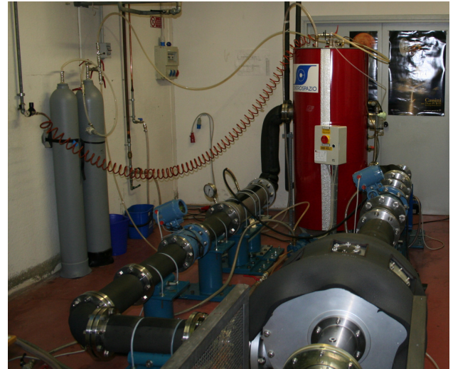
Figure 1 – The Cavitating Pump Rotordynamic Test Facility.
